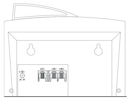
NOTE! Aux input is connected to line 1 and can be used to connect a modem, fax, or ordinary handset type phone. If the Aux input is using line 1, then line 1 will not be available to the system until the Aux call has ended.
